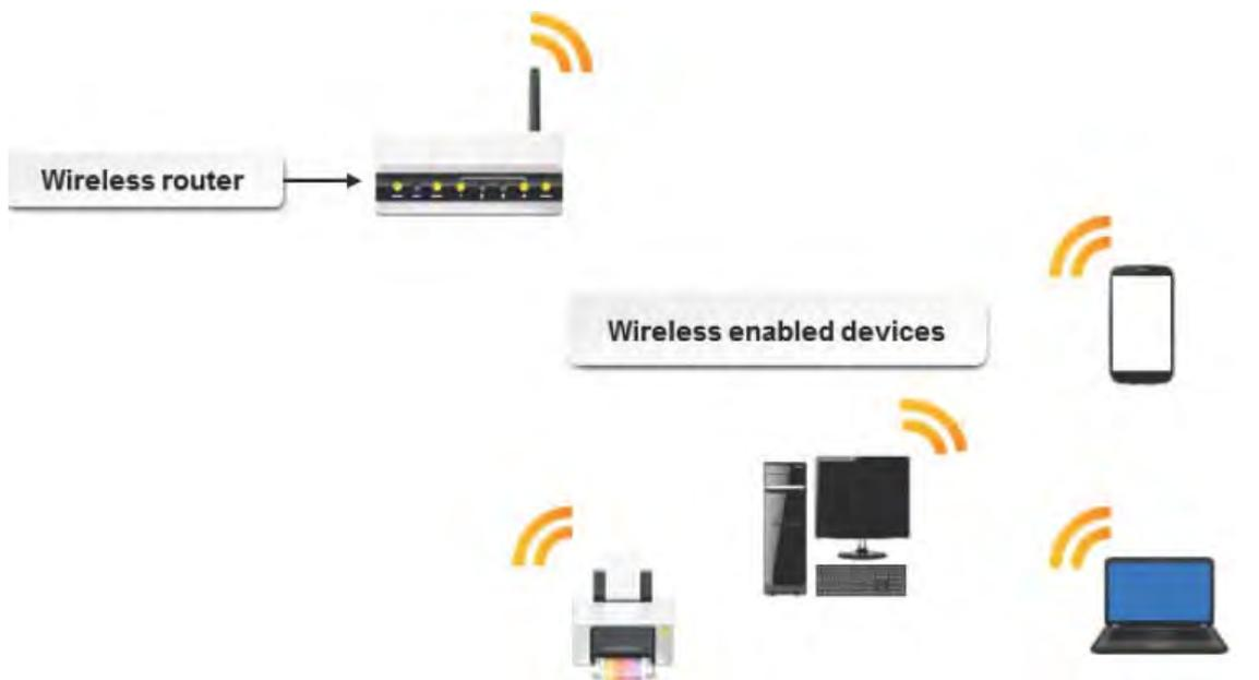
A wireless router connects a computer to multiple networks.
