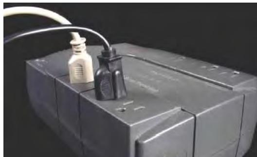
Power connectors connected to a UPS
