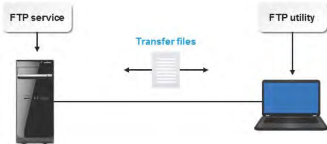
FTP is used to transfer files across a network
